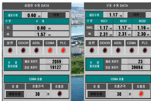
〈Figure 8〉 HMI Monitoring Screen (Gupo and Samrangjin Site)
